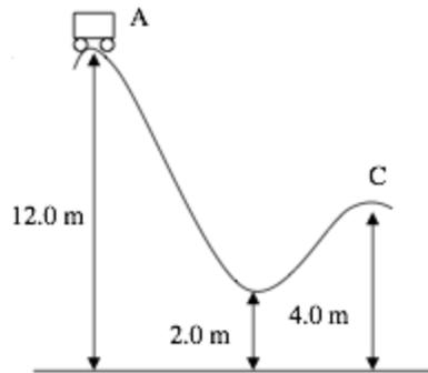
9. The roller coaster shown above has a mass of 525 kg and is travelling at 2.10 m/s at point A, and is later travelling at 12.7 m/s at the lowest point. How much energy was lost to heat on the trip down?
